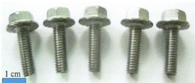
(a) Ultra S.S. 高強度耐腐蝕不銹鋼螺絲(長度約 2.5 cm) Ultra S.S. anti-corrosion screw (about 2.5 cm in length)
