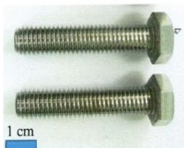
(b) A2-70 不銹鋼螺栓(長度約 5 cm) A2-70 stainless steel bolt (about 5 cm in length)
