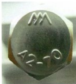
(b) A2-70 不銹鋼螺栓(長度約 5 cm) A2-70 stainless steel bolt (about 5 cm in length)
